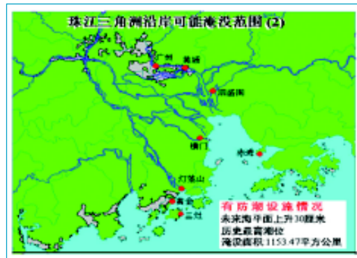
Figure 3.9 The possible submerged area by sea water under the scenario of sea level rise of 30 cm on the condition of the present tide-protecting facilities and the highest historic tidal level in the Pearl River Delta
